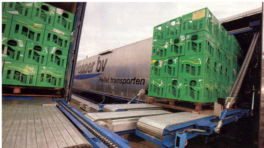
Figure 2 Distrivaart: a conveyor-supported automated compact storage system on a barge (source: De Koster and Waals, 2005).
