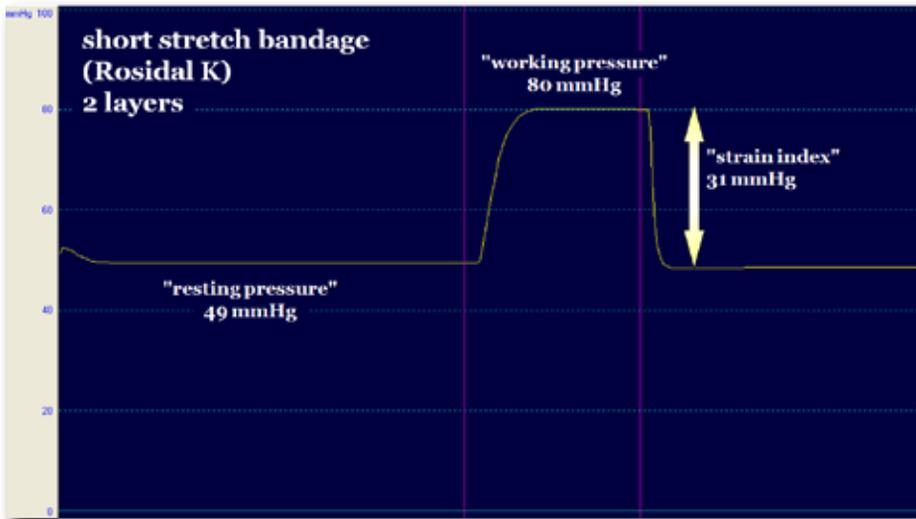
Figure 3.9: a typical recording of the sub-bandage pressure profile on measured on a cylinder; the resting pressure is 49 mmHg, the pressure after inflation to 100 mmHg of the inner sensor is 80 mmHg. The resulting strain index is 31.
