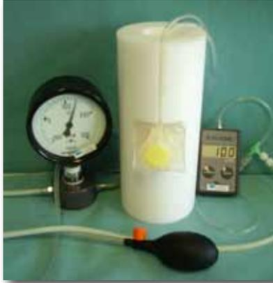
Figure 3.5: the sphygmomanometer connected to the sensor underneath the fluid bag is inflated to 133.33 mbar, which is 100 mmHg pressure on the Kikuhime device.
