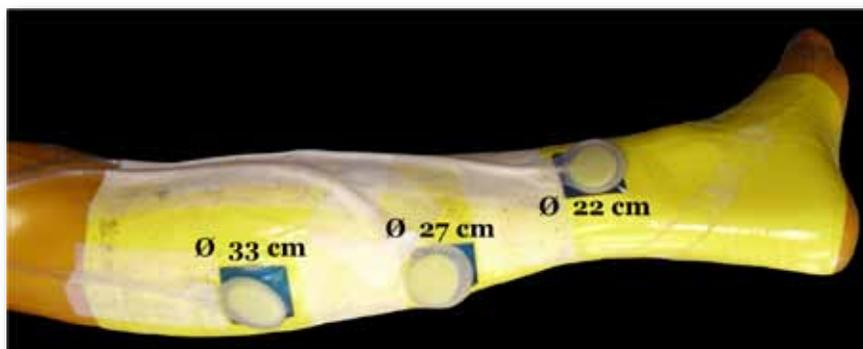
Figure 12.1: artificial leg with pressure transducers at three different circumference levels.
