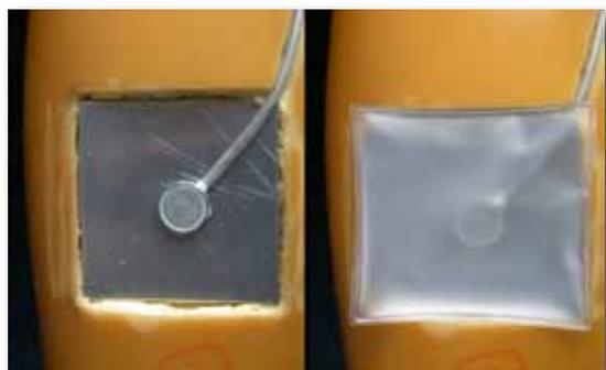
*Figure 5.3.a: positioning of the Gaeltec pressure transducer on top of an aluminium plate.*
