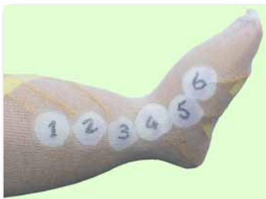
Figure 7.8: the artificial inverted champagne bottle shaped leg with the sensor positioning.
