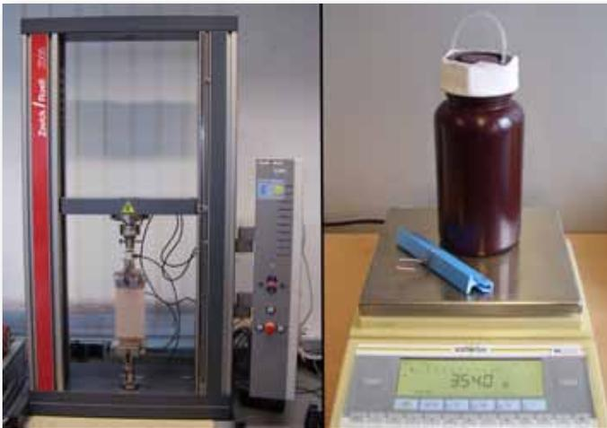
Figure 3.6.a: on a tensile tester, the force e.g. the weight needed to bring each individual component of the compression systems under investigation to the required percentage stretch, was calculated.
