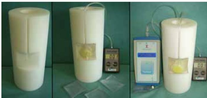
Figure 3.4.a: a poly-oxymethylene test cylinder that can be fitted with a fluid bag and space for sensor tubes without a measurable effect on the final radius of the cylinder.
