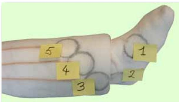
Figure 7.16: artificial leg with skin fold and the positioning of the five pressure transducers.
