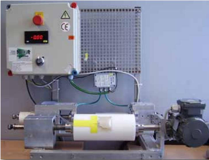
*Figure 3.7: one of the cylinders fitted in the special designed automated roll winder.*
