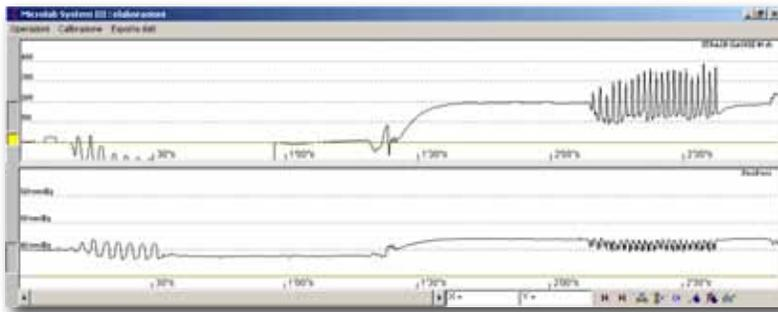
Figure 8.1: simultaneous recording of strain gauge (upper trace) and sub-bandage dynamics (lower trace).
