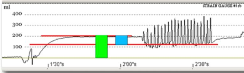
Figure 8.3: strain gauge trace (detail of figure 8.1) showing the venous volume (green box) and ejected volume (blue box).
