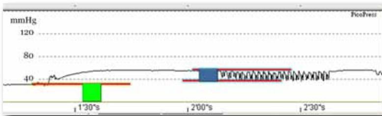
Figure 8.2: sub-bandage pressure measurement (detail of figure 8.1) showing the resting pressure (green box) and working pressure amplitude (blue box).
