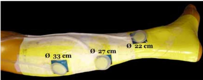
Figure 5.2: artificial leg with pressure transducers at three different circumference levels.
