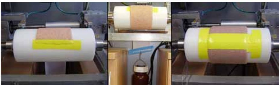
*Figure 3.8.a: the beginning of the bandage is attached with masking tape.*
