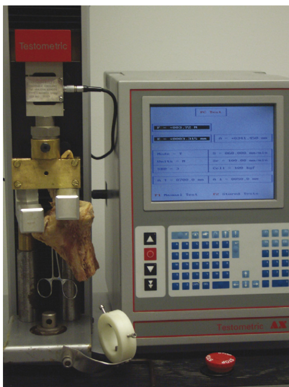
Figure 2. Adjustable testing set up of distraction machine with tibial graft complex fixated.
