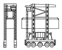
MTS Multi Trailer System (manned). This is a vehicle with five trailers behind it. Is used at the DMU and for transport between stack and rail terminal.
