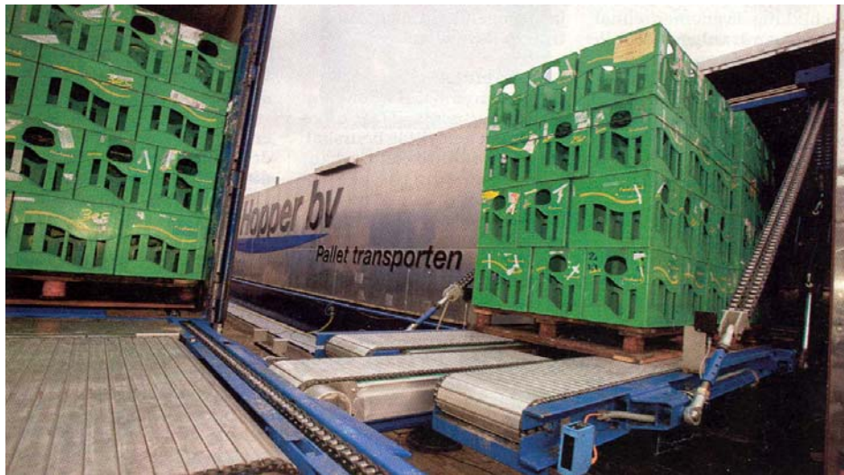
Figure 1: Distrivaart: A conveyor-supported automated compact storage system on a barge (source: Waals, 2005).
