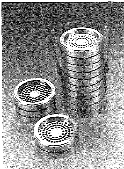
FIGURE 4. Picture of 8-stage Anderson cascade impactor showing the separate stages with progressively smaller orifices.
