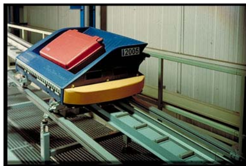
Figure 1 A Destination-Coded Vehicle (courtesy of Vanderlande Industries B.V.)
