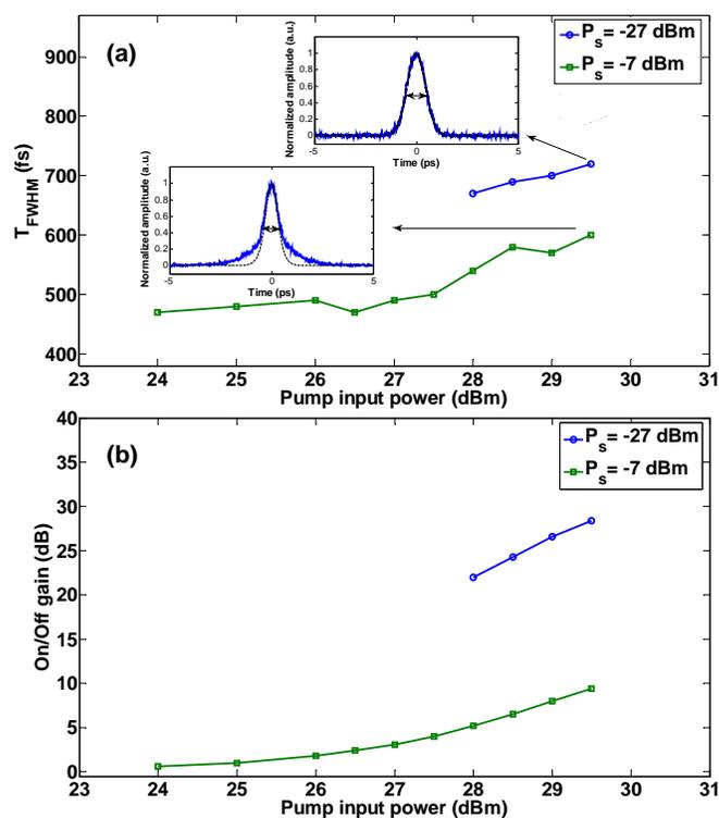
Fig. 2. (a) Pulswidth of the amplified signal as a function of pump power at the input of the HNLF in the saturated ( $P_s = -7$  dBm) and unsaturated ( $P_s = -27$  dBm) regimes. The insets show selected autocorrelation traces. (b) Corresponding measured on/off gain.
