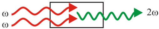
Fig. 1. Principle sketch of second harmonic generation. The generated photons have twice the energy and half the wavelength of the incoming fundamental photons.
