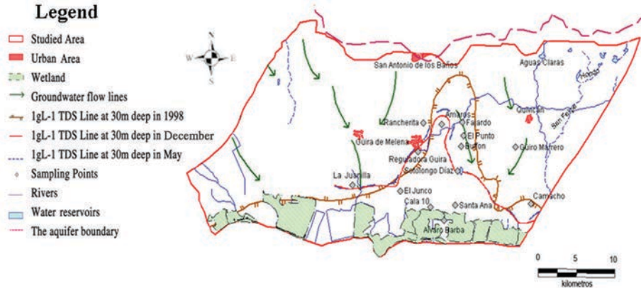
FIG. 1. The hydro-geochemical conceptual model of the aquifer.
