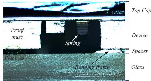
**Figure 13.** Cross-sectional device view from an optical microscope where a dummy device is diced in the middle of the proof mass. Proof mass, electret pattern, and a bonding frame column are seen clearly in the image. A spring connects the proof mass to the bonding frame.
