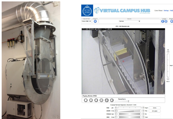
Figure 1: Aerodynamic test facility (left) and camera view on the remote cascade lab module (right).
