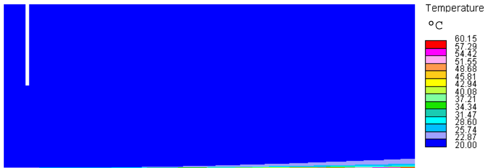
Fig. 5.10 Temperature field in the computational domain corresponding to the experimental configuration in the study of Baughn and Shimizu [39].
