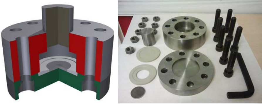
Fig. 3: The device for high pressure nanoimprinting of the nickel foil into the aluminium curved surface. The piston in the top of the device is pressed down in a hydraulic press.
