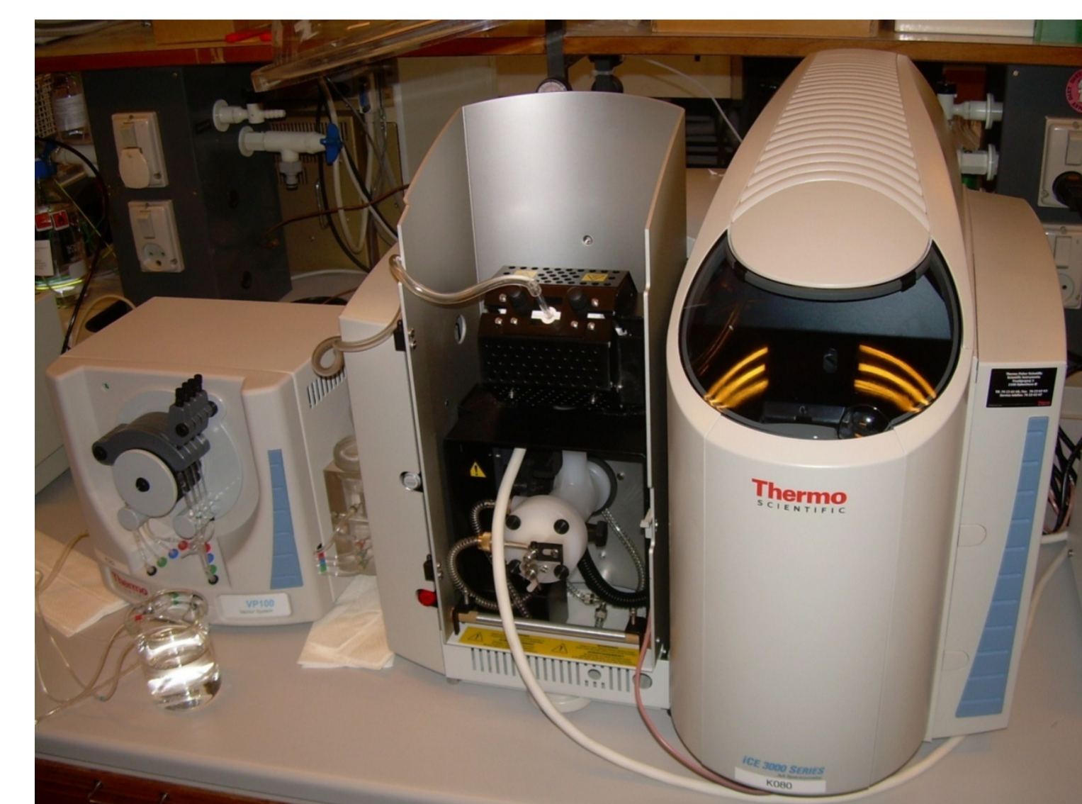
Figure 2. The Atomic Absorption Spectrometer (ICE-3300) coupled with a Hydride Generation system (VP100) and an electrically heated quartz cell (all from Thermo Scientific).
