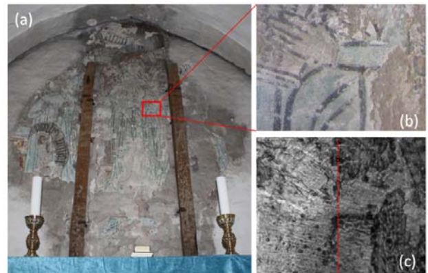
Fig. 1: (a) Apsidal wall painting in Nebbelunde Church - Rødby, Lolland, Denmark. (b) The relevant detail of the painting. (c) THz reflection image of the detail; the red line indicate the scan-line used to image the b-scan shown in Fig. 3.
