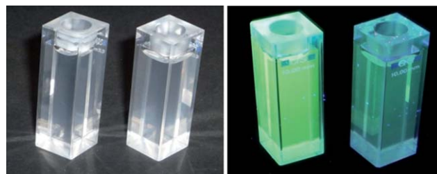
Fig. 6 Photoluminescent emission observation of the nano-particles dispersed in isopropanol under white light (left) and 254 nm (right) excitation. (GA on the left and GP on the right in each image.)
