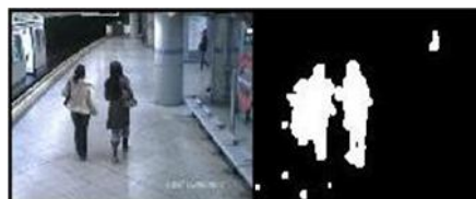
Figure 1. a) current frame b) result of temporal differencing
