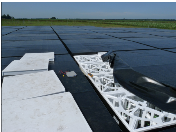
Fig. 7. Left: Closeup image of a single LOFAR HBA tile. The protective covering has been partially removed to expose the actual dipole assembly. The circular dipole rotation mechanism is visible. Right: Median averaged spectrum for all HBA tiles in station CS003. Various prominent RFI sources are clearly visible distributed across the band including the strong peak near 170 MHz corresponding to an emergency pager signal.
