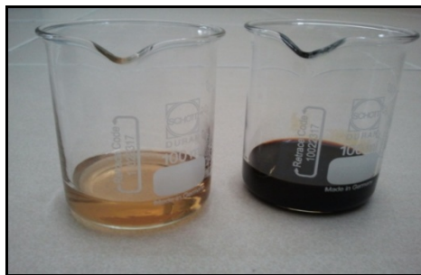
Figure 1: Different colour between fresh (left) and waste (right) engine oil
