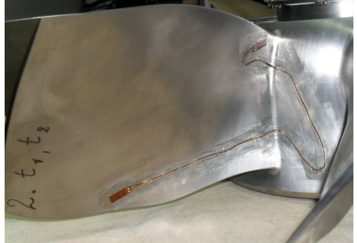
Figure 5: THE INSTRUMENTED STRAIN GAUGES ON THE BLISK1
