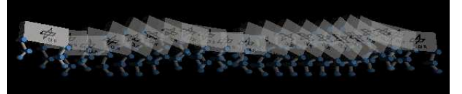
Fig. 8. Image sequence of the forward hopping motion. The picture shows approximately two motion cycles. Thereby, the motion evolves from right to left. For reason of clarity, each image is horizontally shifted by a constant offset.
