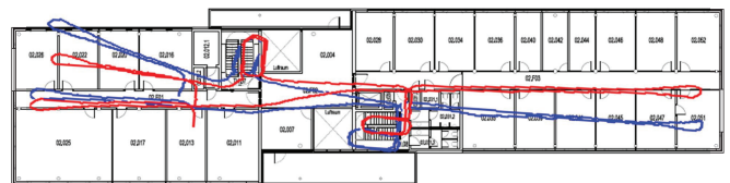
Fig. 18. Odometry for the MTx IMU for the trajectory described in Figure 11. The blue curve represents the output of the data computed using the biases model sampled at 100 Hz and the red line represents the output of the data computed using the model sampled at 200 Hz.
