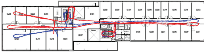
Fig. 14. Odometry for the MTx IMU sampled at 200 Hz for the trajectory described in Figure 11. The blue curve represents the output of the data computed without using the biases model and the red line represents the output of the data computed using the model. In this plot the blue and red curves are completely superposed at the beginning of the walk.
