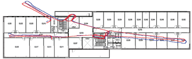
Fig. 16. Odometry for the NavChip IMU for the trajectory described in Figure 11. The blue curve represents the output of the data computed using the biases model sampled at 100 Hz and the red line represents the output of the data computed using the model sampled at 200 Hz.
