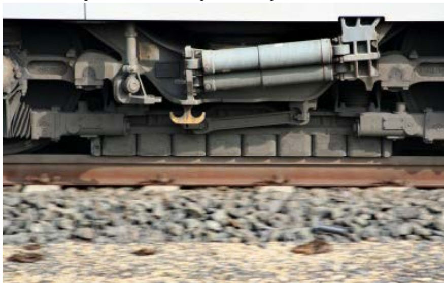
Figure 8: Linear eddy current brake of an ICE 3 in action [25]
