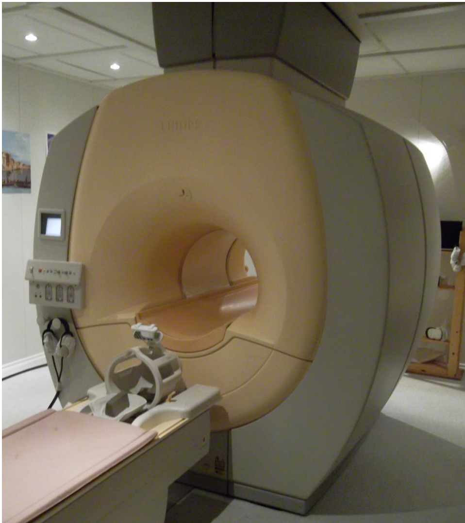
Fig. 4.8: the 1.5 T Philips Intera MR imager at the Exeter MR Research Centre. The SENSE head coil of 8 elements is fixed to the moveable table of the scanner.
