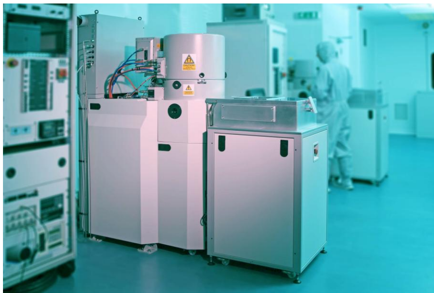
Figure 2.3.1 An example of SPTS Pegasus silicon etch tool. Similar to the tools used in the SPTS locations.
