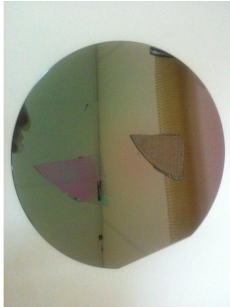
Figure 6.6.1 Carrier wafer with patterned Silicon On Insulator (SOI) coupons fixed to it
