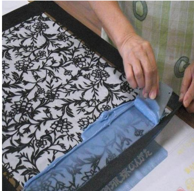
Figure 2.3: “ Kataoki ”: spreading nori (dye-resistant paste) over the patterned stencil to transfer the pattern onto the textile (Photographed at Tamanaha Workshop in Naha)
