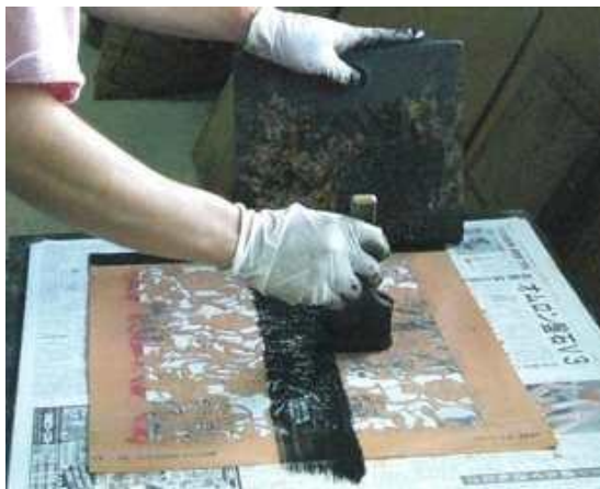
Figure 3.28: Mr. Ashitomi spreading lacquer over the mesh to attach it to the stencil
