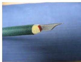
Figure 3.12: The curved and pointed blade of Shigû knife
