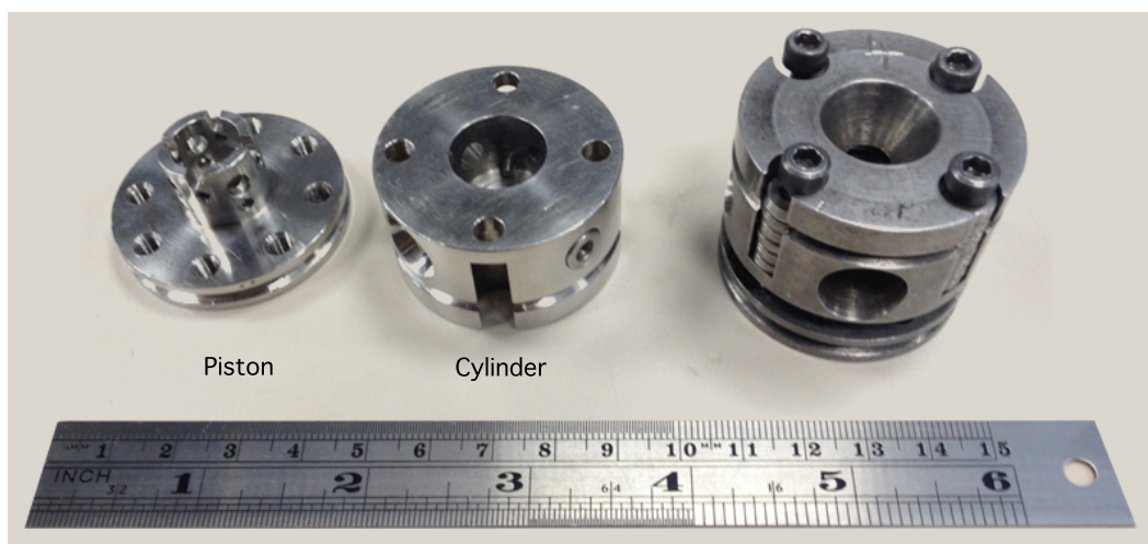
Figure 2.3 Components of a symmetrical screw driven DAC. Four screws (right hand side) are used to drive the piston part into the cylinder part of the DAC.
