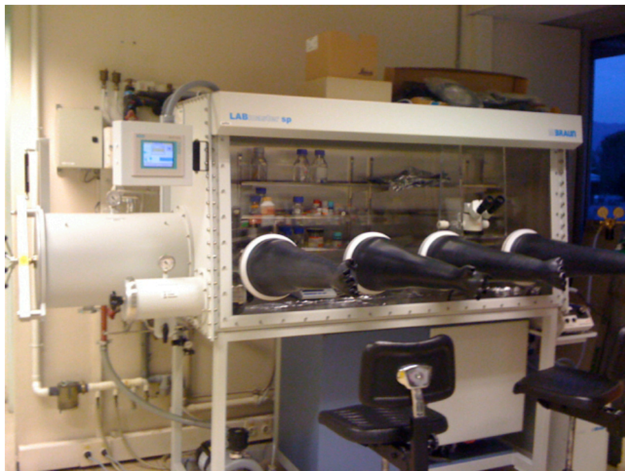
Figure 2.14 Glovebox at the ESRF. The right hand side of the box shows the DAC loading area (built in microscope).
