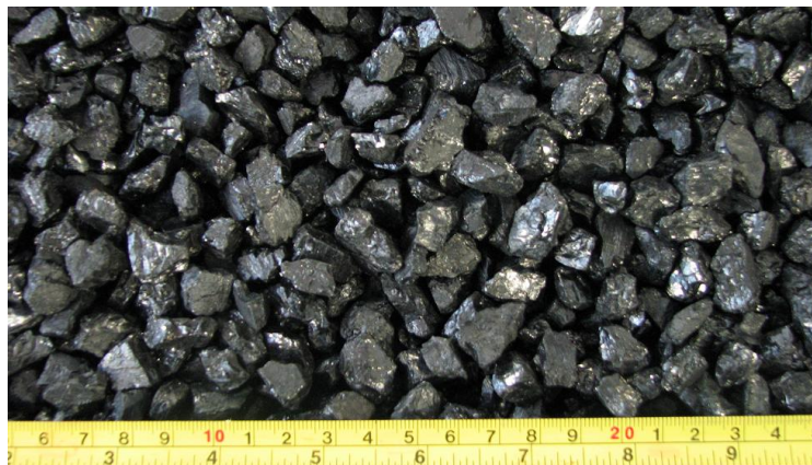
Figure 8.5: Close up view of the granular bed consisting of anthracite rocks.
