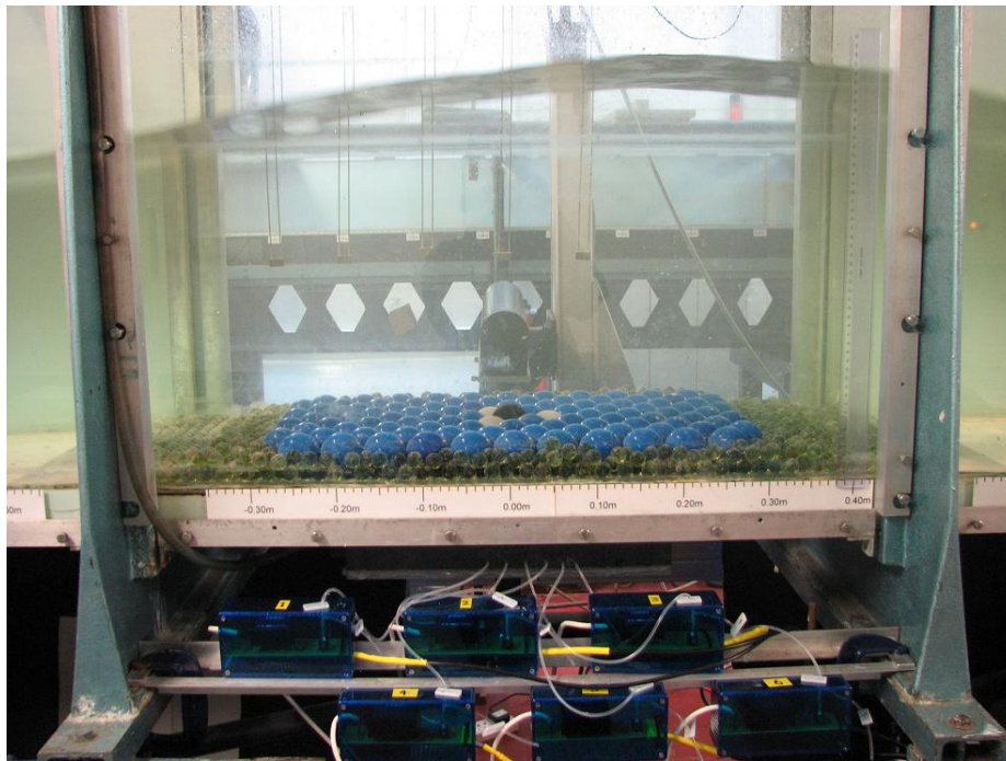
Figure 3.13: Waves running over the rough bed. Pressure tappings are connected to Honeywell 40PC001B2A type pressure sensors housed in the boxes below.
