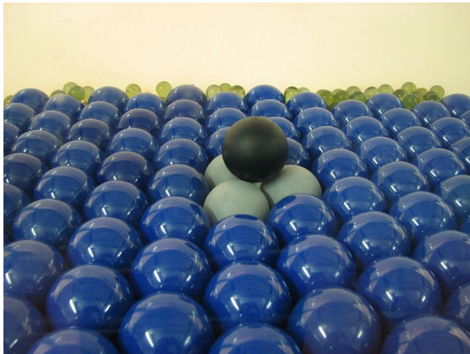
Figure 3.8: Measuring sphere (black) over the rough bed of 50mm billiard balls.
