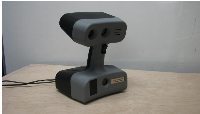
Figure 3.31: Artec scanner used for 3D scanning to obtain a digital surface elevation map of the model bed protection.
