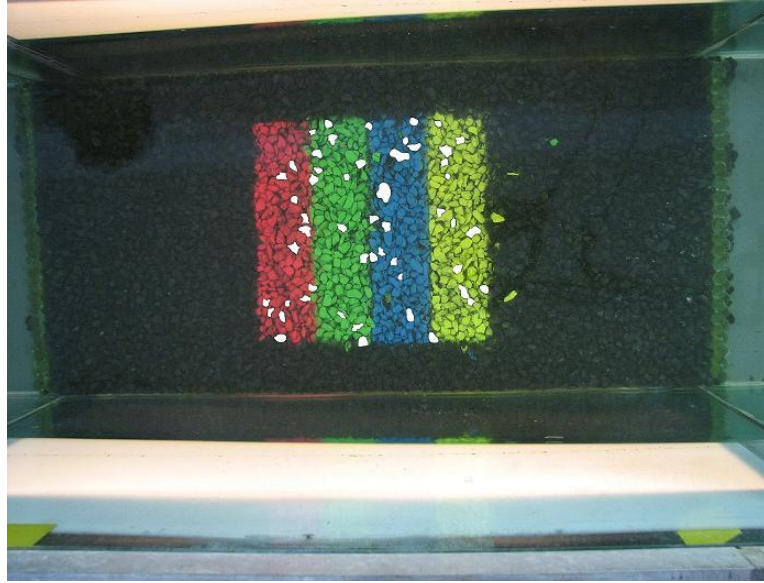
Figure 3.56: Damage to a model bed protection – rock count.
