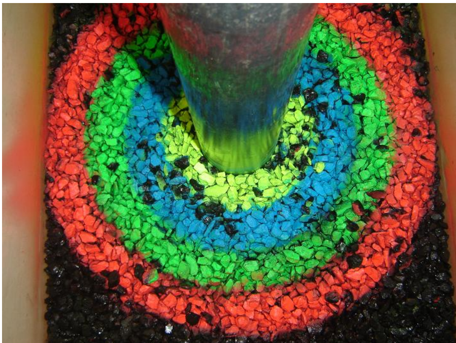
Figure 8.20: Bed protection around a monopile before the start of model run.
