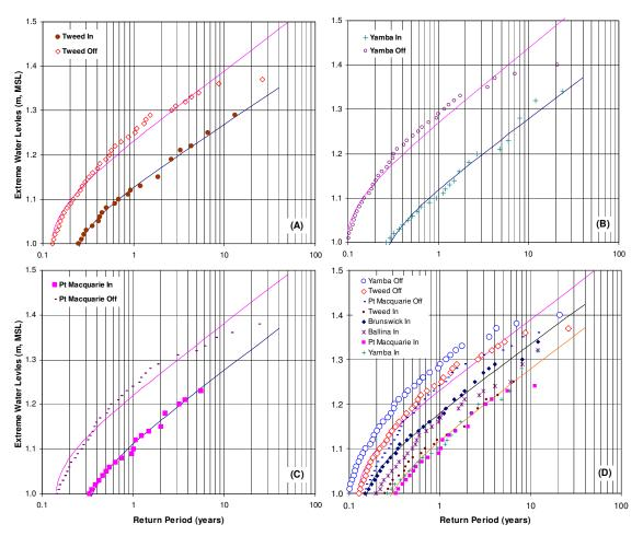
Figure 6:Comparison of the empirical distributions of extreme water levels measured on the northern NSW coast at: [A] the paired inshore and offshore sites of the Tweed River entrance; [B] the paired inshore and offshore sites of the Yamba River entrance; [C] the paired inshore and offshore sites of the Port Macquarie River entrance; and [D] the river entrances and offshore stations, where the solid line is the FT-I distribution fitted to the offshore and river entrance data.
