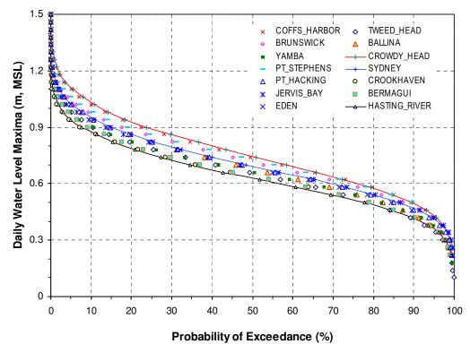
Figure 3: Distributions of daily water level maxima computed from the 14 inshore stations. The daily water level maxima at the stations (Crowdy Head and Eden) directly exposed to ocean waves are generally larger (~5cm) than those inside the bays or harbors (Sydney, Pt Stephens, Port Hacking, Jervis Bay), and about twice larger (~10cm) than those at the trained river entrances, excluding the Brunswick River entrance.
