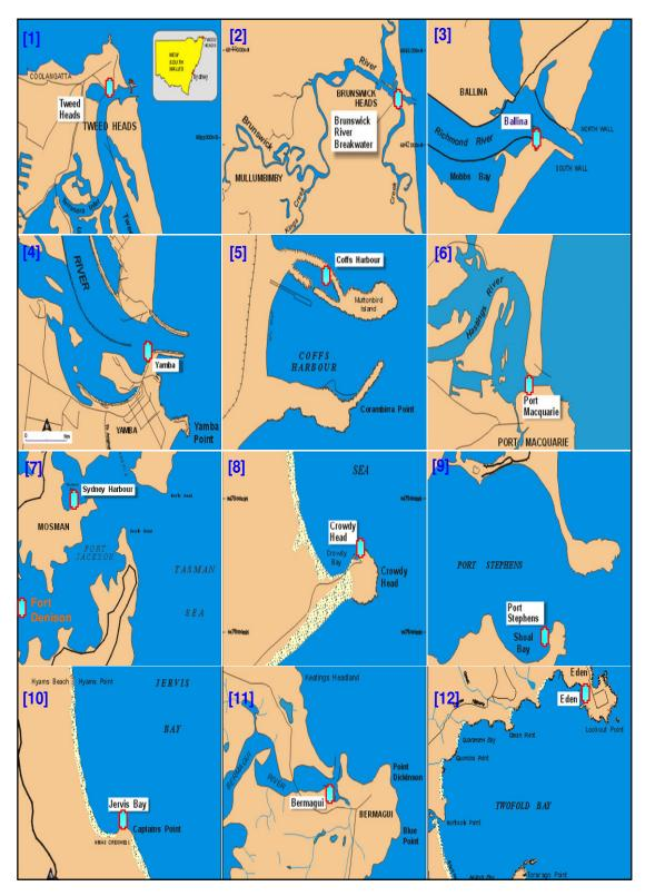
Figure 2: Location maps of the 12 inshore tide gauges deployed at the river entrances [1, 2, 3, 4, 6, 11] and inside the bays [8, 9, 10, 12] and harbors [5, 7] along the Australian East Coast of NSW. Note the upward/downward direction of the location maps is the north/south.
