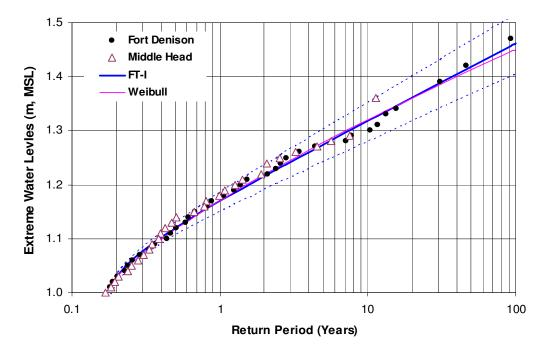
Figure 7: The FT extreme-value distribution is applied to estimate *n*-year return water levels from the monthly maximum water levels collected at Fort Denison inside Sydney Harbor, where the data at Middle Head inside the same Harbor are plotted for comparison, where the Weibull is also included.
