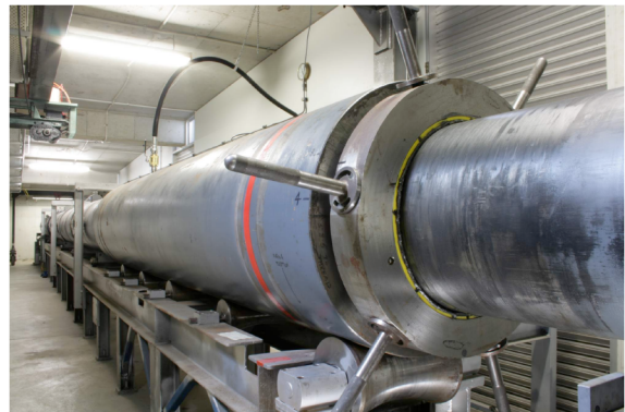
Fig. 4. X3's upgraded free-piston driver. Bore is \varnothing 500mm.
