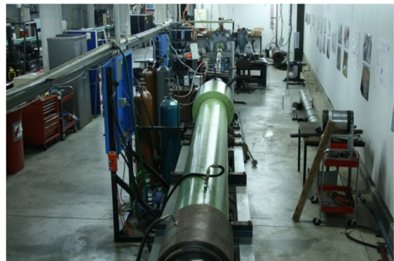
Fig. 3. Photograph of X2; compression tube is shown in the foreground; acceleration tube and test section is shown in background.
