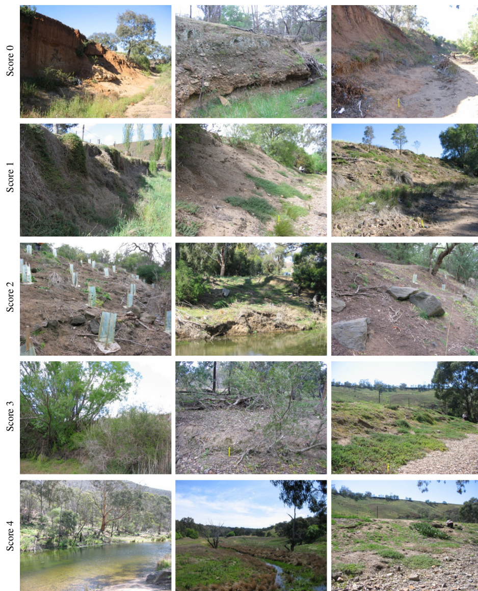
Fig. 2 Field photos of different levels of bank condition in relation to the Index of Stream Condition (Ref. 10).
