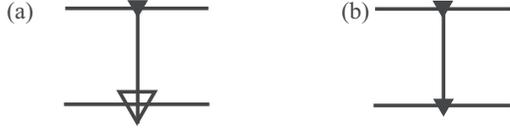
FIG. 1. (a) Circuit representation for the controlled-double-NOT gate  $\nabla(X)$ . The control (target) ququart is denoted by the closed (open) triangle. (b) Circuit representation for the controlled-double-phase-flip gate  $\nabla(P)$ .
