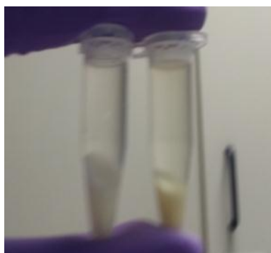
Figure 17 : Gastric (left) and intestinal (right) aliquots after in vitro digestion. As can be seen, the precipitate includes not only iron. What is referred to as precipitate iron is both normal precipitated iron and also whatever iron is caught in this yellow precipitate.
