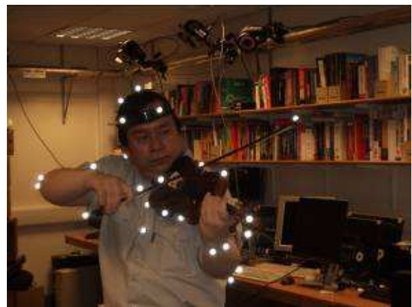
Figure 3. A photo of a motion capture session with the markers highlighted.
