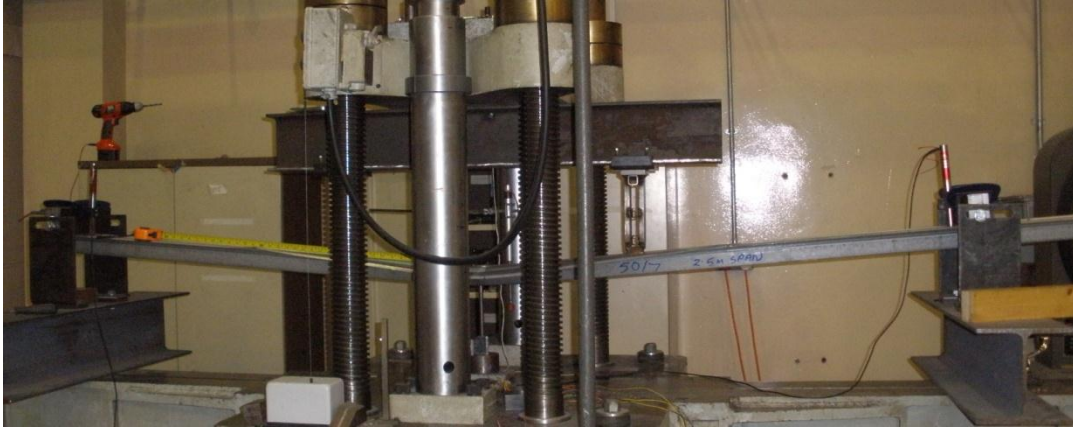
(c) Test photograph of uplift loading direction for U-61-N3 specimen
