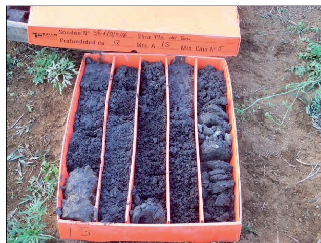
FIGURE 4 | Field photograph of the pyroclastic level. Located on top of the level of dated silts and clays.
