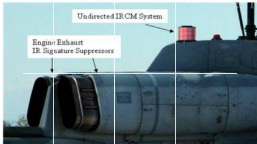
Figure 3-13: AH-1 IRCM Installation and IR Signature Suppressors – (U.S. DoD Photo).
