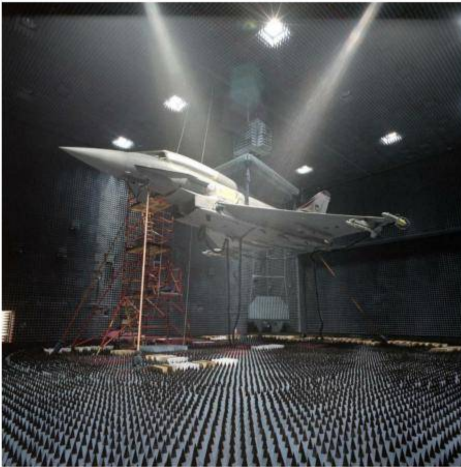
Figure 6-7: ISTF Example 2: EW Test Facility – (© BAE SYSTEMS 2010, All Rights Reserved).
