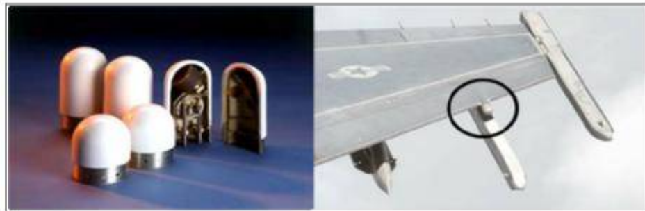
Figure 2-9: a) Uninstalled RWR Antennas – (Courtesy L3 – Randtron Antenna Systems); b) Installed F-16 RWR Antenna – (U.S. DoD Photo).
