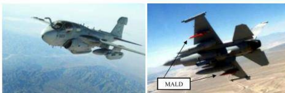
Figure 3-8: a) EA-6B Aircraft with External Jamming Pods; b) Miniature Air Launched Decoy Carried by F-16 – (U.S. DoD Photos).
