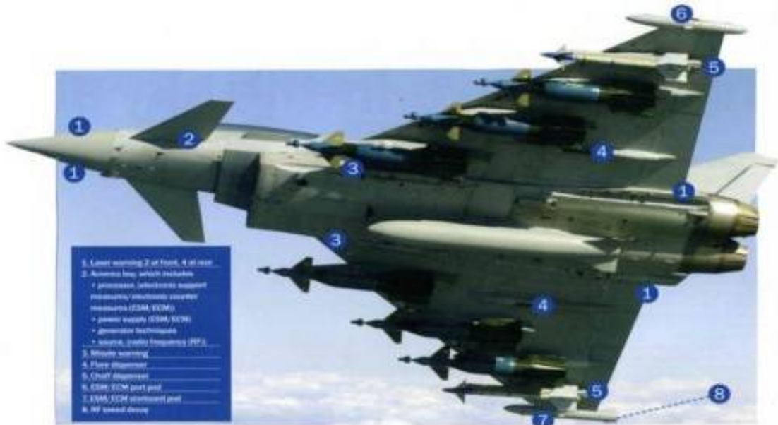
Figure 6. DASS equipment locations on Typhoon. (© BAE Systems 2009, all rights reserved)
