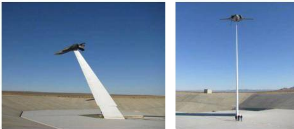
Figure 3-26: F-35 Model Undergoing RCS Measurements – (Lockheed Martin Photos).
