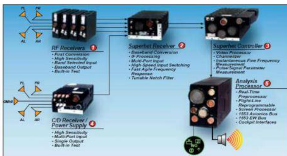
Figure 2-7: RWR Components and Functions – (Courtesy of BAE Systems).
