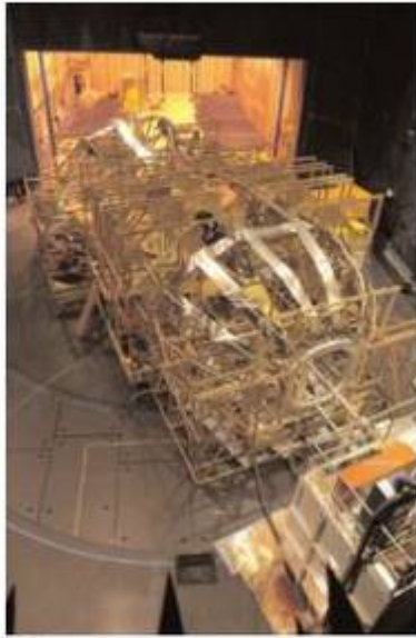
Figure 16. Lightning strike testing in EWTF anechoic chamber.
