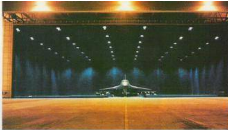
Chambers such as the US Air Force's Benfield Anechoic Facility, above, can provide a sterile RF environment for more effective EW testing. (US Air Force photo)
