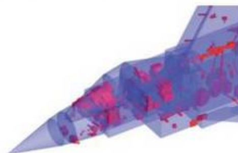
Figure 6. Quantitative vulnerability modeling – example selection of components. Reproduced from BAE Systems © 2009.
