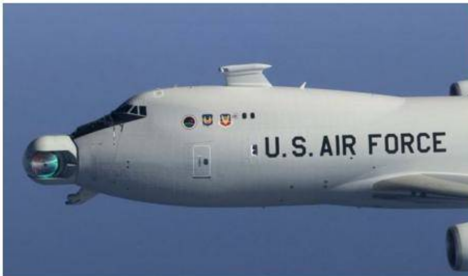
Figure 3-29: The YAL-1 Airborne Laser System – (USAF Photo).
