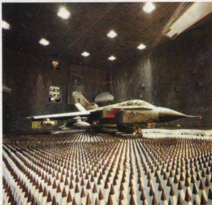
A Royal Air Force Tornado undergoes testing at the British Aerospace EW test facility. (British Aerospace photo)
