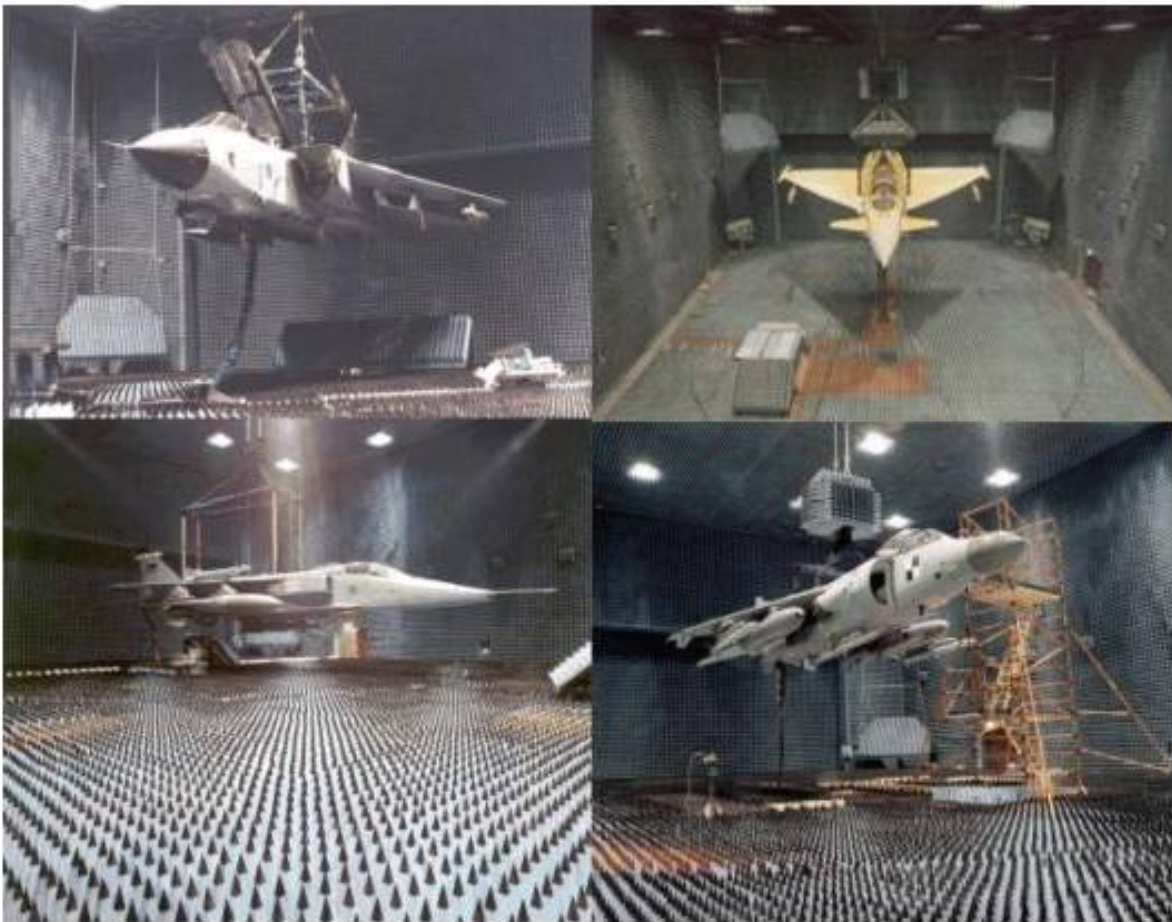
Figure 20. Selection of aircraft tested in EWTF chamber. (© BAE Systems 2009, all rights reserved)
