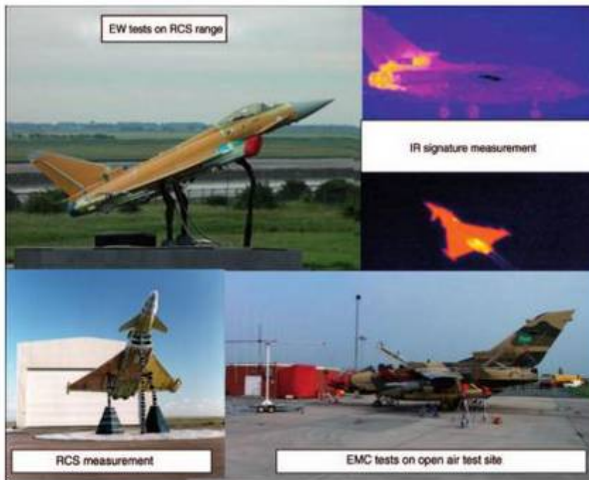
Figure 9. Measurement facility examples. BAE Systems © 2009.
