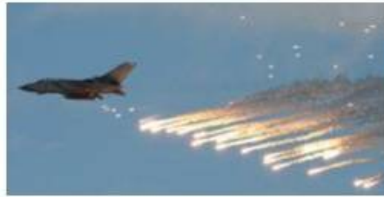
Figure 8. Flare dispensing from AIRCM pod. (Unknown ‘spotter’ photograph from Internet)
