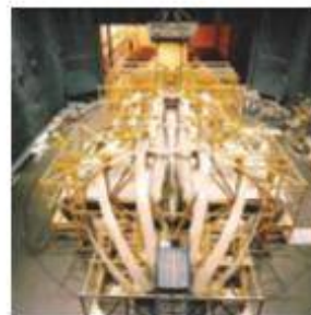
Fig. 3 Typhoon in lightning-strike tests.
