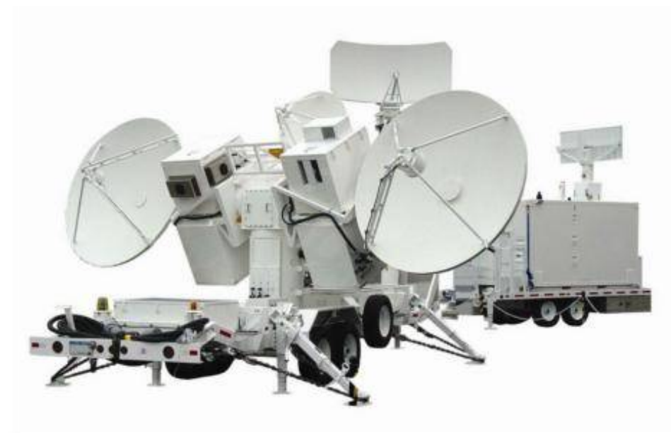
Figure 6-9: Typical Range Threat Simulator – Joint Threat Emitter (JTE) – (© Northrop Grumman Amherst Systems Inc.).
