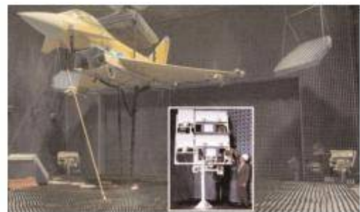
Figure 5. Radiated EW tests in anechoic chamber. (© BAE SYSTEMS)
