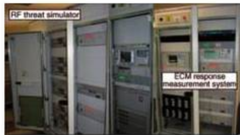
Figure 8. RF threat simulator and ECM response measurement system. Label 1: RF threat simulator; Label 2: ECM response measurement system. BAE Systems © 2009.
