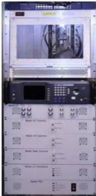
Figure 22. Chameleon II radar target and ECM simulator. (© EWsT, a Herley Company, 2009)
