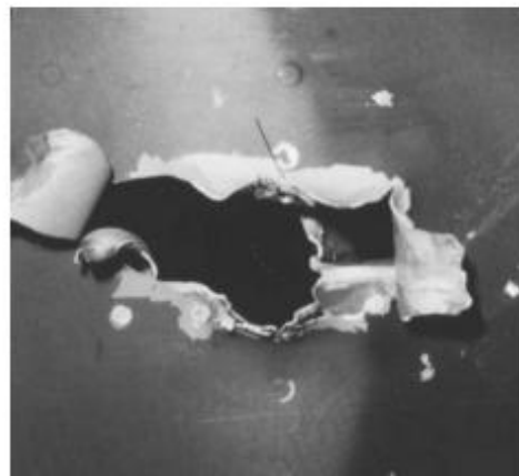
Figure 2. Example of metallic structural damage. Reproduced from BAE Systems © 2009.
