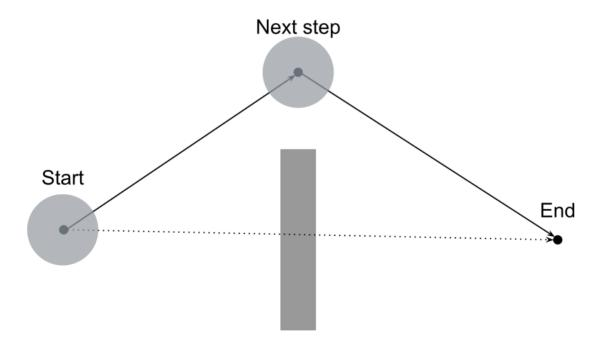
If there wasn't for the wall on the way the robot could simply set its next destination to the end point and drive there. Now we have to take more steps to arrive at the end. To keep our solution as general as possible we only output the next step to be taken by the robot.
