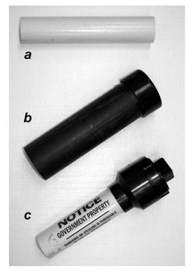
FIGURE 1. Brown tree snake (*Boiga irregularis*) bait station types tested in this study. a, "2 by 12" station, placed horizontally, both ends open. This is the station type used most widely on Guam for operational snake eradication; b, "4 by 12" station, placed at  $\sim 45^\circ$  angle, lower end open; c, "C-O" station, placed at  $\sim 60^\circ$  angle, lower end open.
