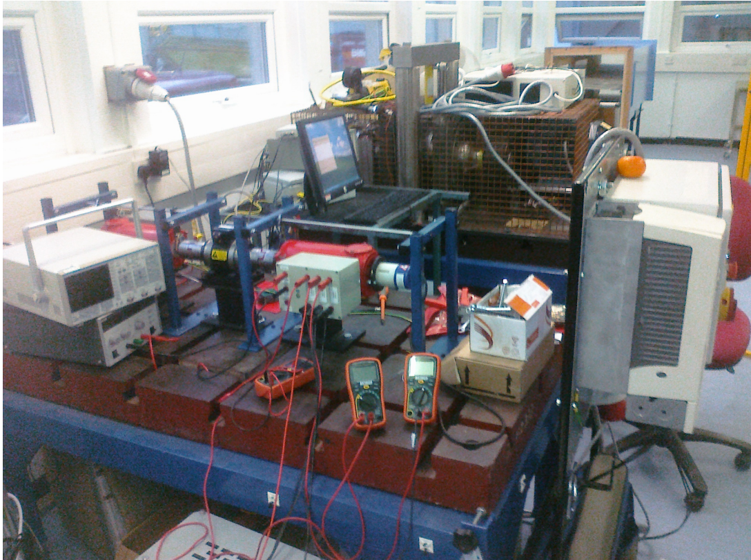
Figure 8.6: Photograph of the bearing current test rig
