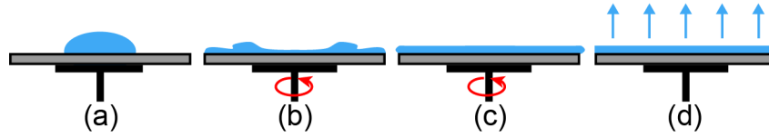
Figure 3.8: Schematic diagram showing spin-coating, adapted from [10].
