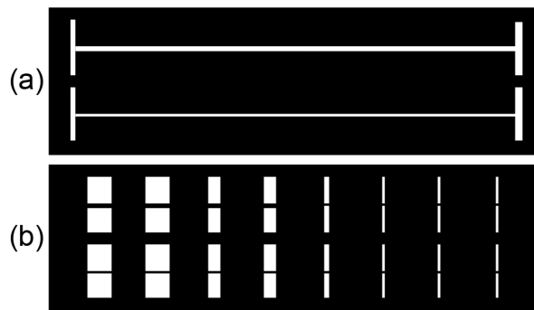
Figure 9.1: Shadow masks used for evaporating (a) aluminium gate and (b) gold source and drain electrodes
