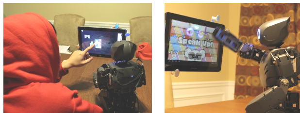
Figure 1. A cognitive robotic system is coupled with an Android toolkit that transforms a tablet into a shared workspace for engaging and learning a task during human-robot collaboration.
