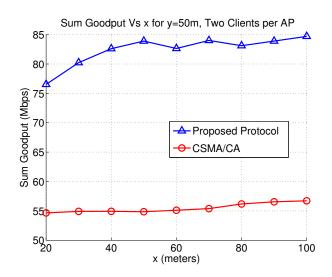
Fig. 8. Sum goodput as a function of x for y = 50 meters for the topology shown in Figure 7, where each of the two APs have two clients.
