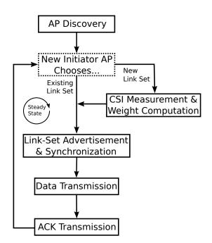
Fig. 2. High level flowchart of proposed protocol. Phases are shown with solid borders.
