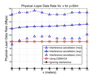
Fig. 9. Data rate for two OBSS with a single client in each BSS.
