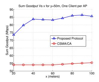
Fig. 6. Sum goodput as a function of x for y = 50 meters for the topology shown in Figure 5, where each of the two APs have a single client.
