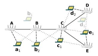
Fig. 1. A five AP example highlighting the AP topology (solid lines) and an example link set (dashed lines) with the interference that can be cancelled (dotted lines).
