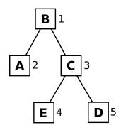
Fig. 4. Tree structure of five AP example showing an example round-robin order as chosen by the worker AP.
