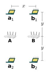
Fig. 7. Topology of two OBSS where each BSS has two clients.
