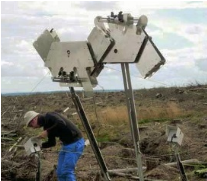
Right: The Bartlett team set up the cells with their own power sources and solid state recording technology so that they would run much like a probe to another part of the solar system
