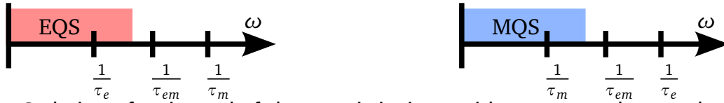
Figure 2.1.: Ordering of reciprocal of characteristic times with respect to the angular frequency. Source: [37]
