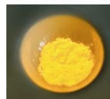
further treatment was achieved. PSD and SEM measurements confirmed the formation of nanocrystalline phosphor crystallites. These compounds with spherical shaped particles exhibit comparable luminescence properties to commonly synthesized 2-5-8 compounds. Sintering of the nanocrystalline solid solution compound (Ba<sub>1.5</sub>Sr<sub>0.5</sub>Si<sub>2</sub>N<sub>5</sub>:Eu<sup>2+</sup>) leads to translucent Lumiramic<sup>TM</sup> ceramics with a phosphor particle size of 500 nm.
