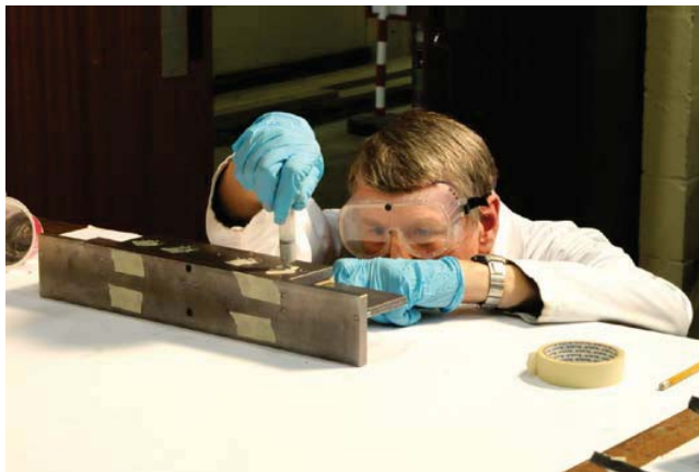
Injection process for test specimen using an in-house bolt location jig.
