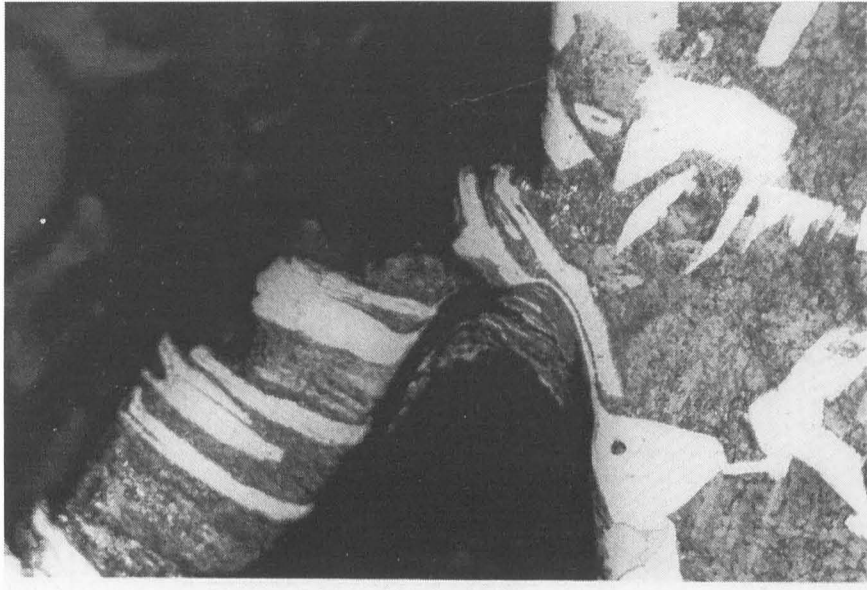
Figure 4.55 Optical microscope view of section through quick stop sample for 30m/min and 0.05mm/rev, dry, 300x.
