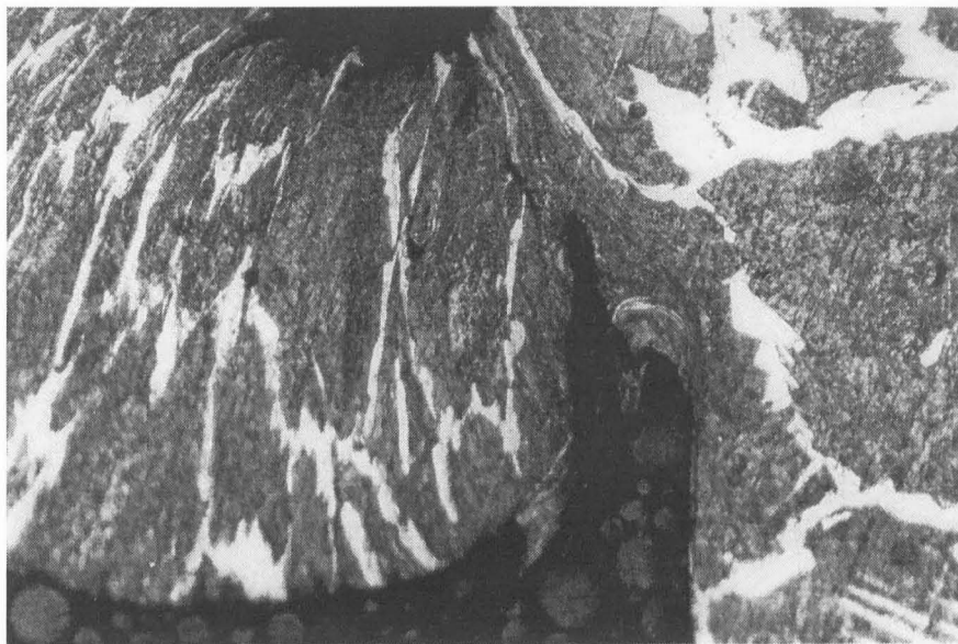
Figure 4.53 Optical microscope view of section through quick stop sample for 22m/min and 0.15mm/rev, 0%, 150x.
