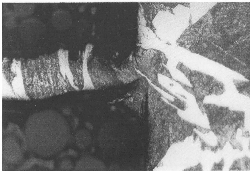
Figure 4.65 Optical microscope view of section through quick stop sample for 40m/min and 0.05mm/rev, 0%, 300x.
