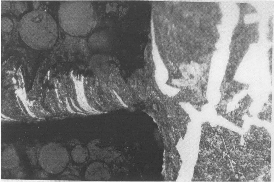
Figure 4.61 Optical microscope view of section through quick stop sample for 30m/min and 0.15mm/rev, dry, 300x.
