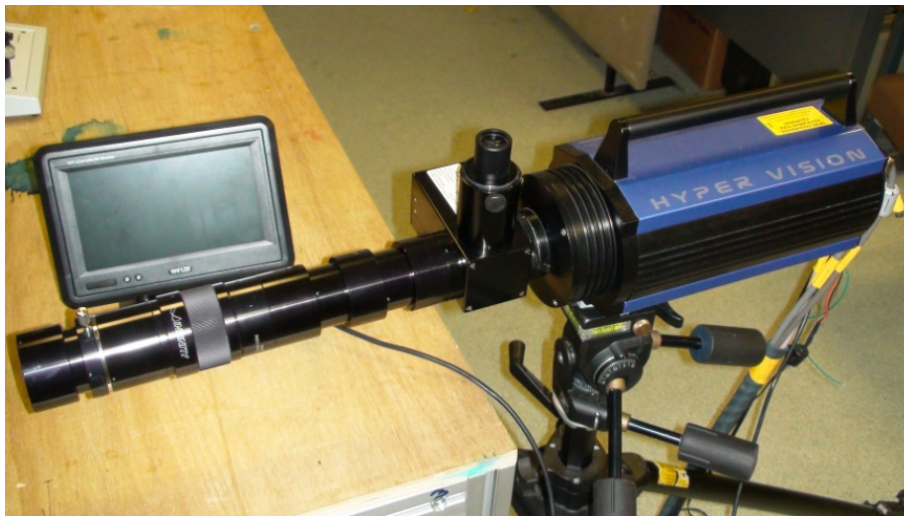
Fig. 4.3 High speed video camera with K2 long distance microscope
